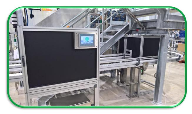
28800 products pass through the device per shift which can be processed by the cameras without trouble. The PLC programme provides statistics on the display of HMI about the Good, Faulty, Not Read and All products. These statistics and the signal of the tower light make clear for the operator if there is a production problem and decrease the time spent on solving the problem thus minimizing waste production.
